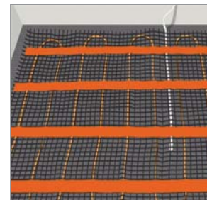
Floor sensor must be placed under the mat between two heating cables
