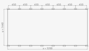
H1. Max. Design wind load: 2.0 kN/m<sup>2</sup>
