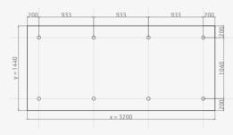
H1. Max. Design wind load: 1.5 kN/m<sup>2</sup>
