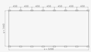
H1. Max. Design wind load: 2.8 kN/m<sup>2</sup>
