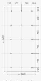
V2. Max. Design wind load: 3.0 kN/m²
