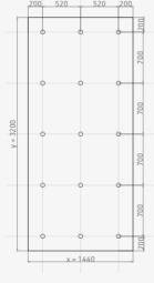
V2. Max. Design wind load: 3.0 kN/m²
