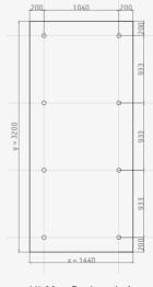
V1. Max. Design wind load: 0.5 kN/m²
