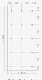
V2. Max. Design wind load: 1 kN/m²
