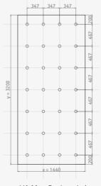
V4. Max. Design wind load: 2 kN/m²
