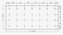
H4. Max. Design wind load: 5.5 kN/m<sup>2</sup>
