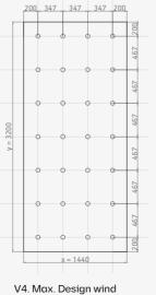
V4. Max. Design wind load: 5.5 kN/m<sup>2</sup>
