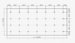
H4. Max. Design wind load: 5.5 kN/m<sup>2</sup>
