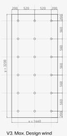
V3. Max. Design win load: 3.5 kN/m<sup>2</sup>
