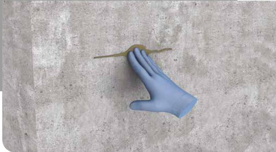
When mixed with clean water and applied correctly it is formulated for the rapid patching and plugging of active water leaks and seepage in concrete and masonry.
