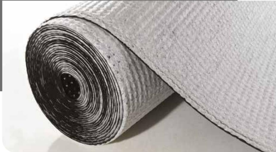
The dual layers comprise of the Wykamol 8mm studded HDPE membrane and a non-woven geotextile manufactured from UV stabilised, virgin polypropylene fibres that have been mechanically entangled to provide high strength, high extensibility, high loft and excellent abrasion characteristics. The geotextiles are also thermally treated to reduce thickness while maintaining excellent mechanical properties.
