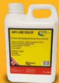
Wykamol Anti-Lime Sealer is a highly penetrative solution specially formulated to react with hydrated cement both at the surface and to a depth of up to 15 mm. The Silicate active ingredients form monolithic structures within the concrete which are long-lasting and durable and will improve surface wear characteristics.
