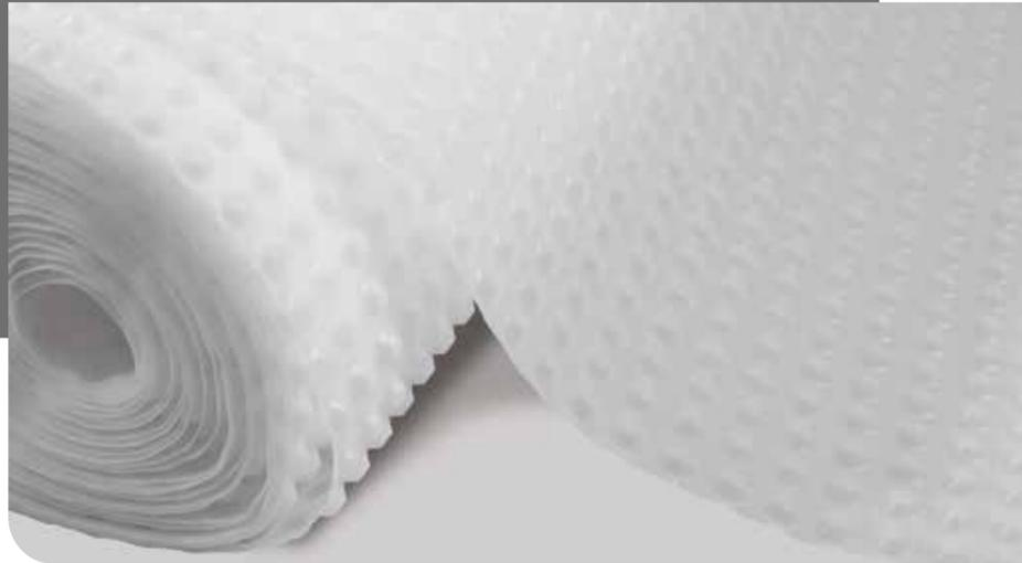
CM8 Cavity Drain Membrane is an 8 mm studded membrane, suitable for Type C waterproofing and delivering a grade 3 environment to BS8102:2022 and NHBC Chapter 5.4. CM8 is available in both 500g or 700g densities. We recommend using the CM8 HD700 when a heavier, denser membrane is deemed necessary by the Wykamol Technical Department or when a Radon barrier needs to be incorporated. Please always take advice from our Technical Experts when making product selections.
