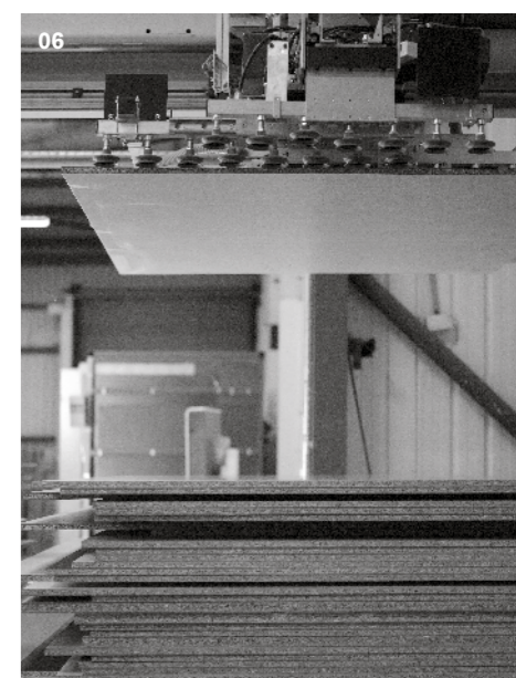
06 Recycling Robotic handling systems ensure maximum board utilisation is achieved
