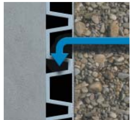
Drainage sheets with a welded-on geotextile form a seepage layer which ensures that any water influx drains away safely.
