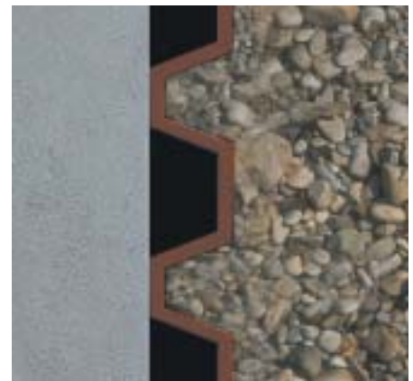
Common dimpled sheets get clogged up with soil and lose their drainage function.
