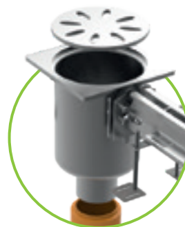
BG-OMEGA outlet elements incl. odour trap and sediment bucket, vertical outlet
