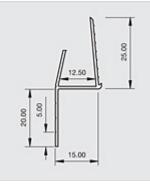
Locally manufactured from recycled plastic, Renderplas PVCu architrave shadow gap beads are designed for plasterboard to quickly and accurately
