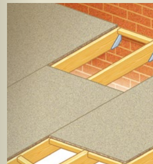
SE panels are laid with long edges in-line with the joists
