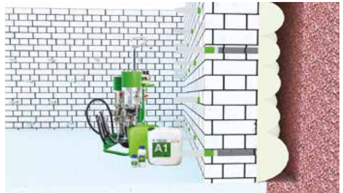
Curtain Injection of Masonry
