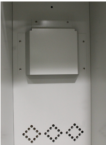
Electronic ventilator for active air exchange
