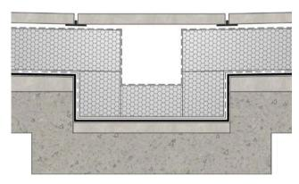
Figure 6. Ballasted inverted roof - insulation over internal gutter
