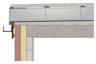
Figure 7. Ballasted inverted roof – detail at eaves
