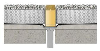
Figure 4. Ravatherm XPS X MK system in the inverted roof
