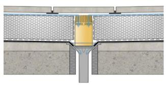
Figure 5. Ballasted inverted roof – outlet protected by paving slabs
