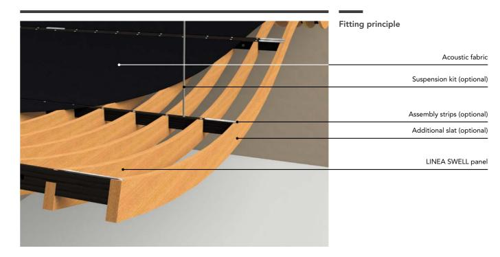
Edge finishing by adding an additional slat (option) attached with assembly strips (option).
