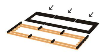
Step 5: Fix the particle plates on the slats
