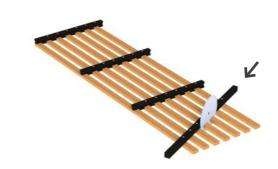
Step 3: Screw on the profile to hold the slats
