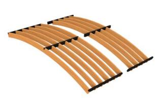
Step 3: Panel ready to be fitted, after drilling the counter-slats for the hangers (Ø 9 mm)
