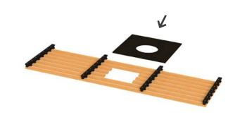
Step 5: Fix the particle plate on the slats
