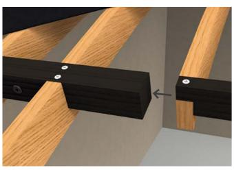
Step 2: Assemble the panels using the assembly strips and 4 screws
