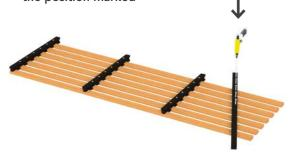
Step 4: Cut the panel along the cutting profile
