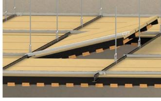
Step 4: The spacer bar is unclipped
