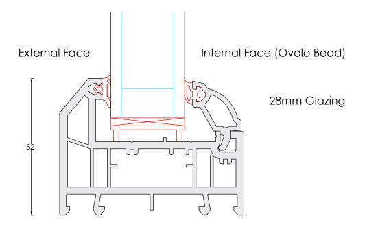
Not used as a door outer frame only used as a low PVCu threshold
