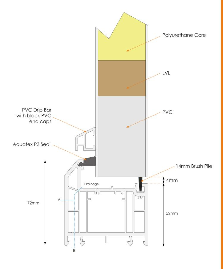
A= Face Drainage (Slots 5mm x 35mm)
