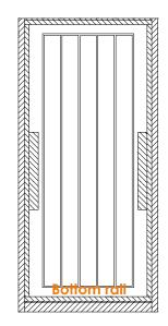
Door sashes less than 1896 in height cannot have a letterplate fitted in the bottom rail.
