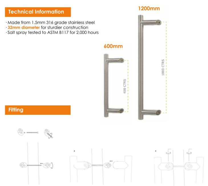
Suitably line the holes up to where the handle will be fitted on the door making sure it is straight. Take 'fitting A' and feed through the bolt. Screw 'fitting B' onto the other side. Push each handle onto its fixings.
