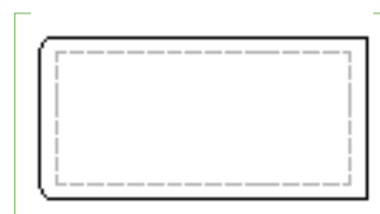
End unit: Rounded corners one end; square-faced one end. Used as end modules on multiple unit seating runs.
