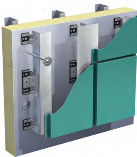
Fixed through composite panel
