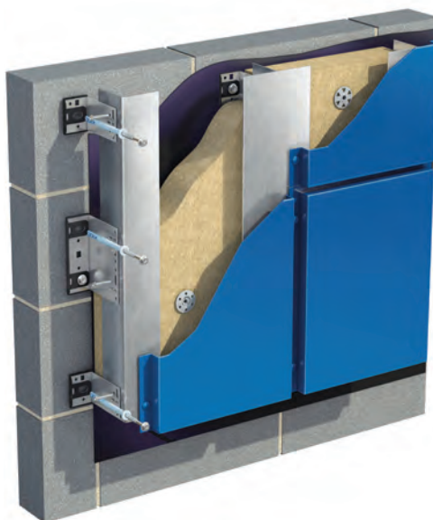
Fixed to masonry
