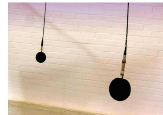
A number of suspended microphones to determine the special average sound pressure level of a room.
