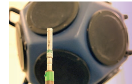
Dodecahedron speaker used in laboratory and field measurement of sound insulation and reverberation times in conjunction with a level monitoring microphone.
