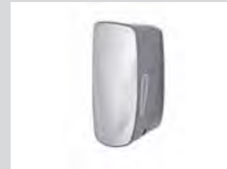
Liquid soap/foam dispenser Light Grey plastic Wall mounted dispenser for liquid soap/foam. Light Grey ABS case and stainless steel cover with 900ml refillable reservoir. H255 x W130 x D120mm Code: 0302513/0302514
