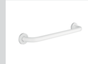
Grab rail White aluminium Aluminium grab rail 600mm long with white polyester coated finish and concealed fixings. W600 x D95 x Ø35mm Code: S6454AC
