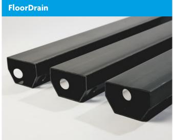
The Wykamol Floor Drain Drainage Channel is a PVC drainage conduit for the control of water ingress in below ground waterproofing situations. Wykamol Floor Drain is flangeless (no up-stand) and can be fitted across the centre of the basement floor, directing any ingress of water towards a sump chamber or drain.
