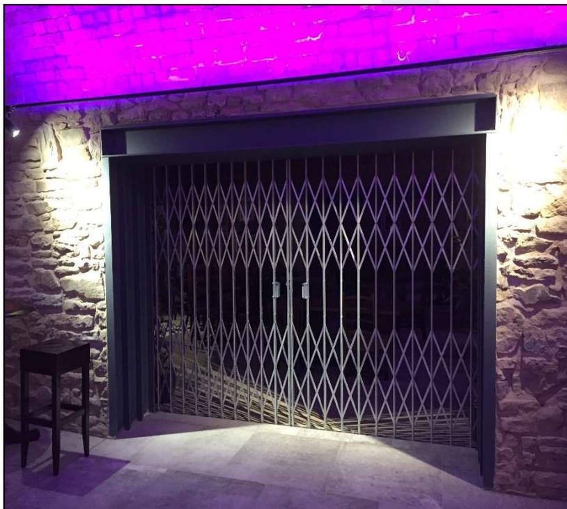
Spearhead gates run on a flat bar bottom track which is folding or portable. The top track is a folding or portable flat bar. The weight of the gate is supported by pulleys at the base of the pickets. Pairs are supplied with removable centre post and fixing stay.
