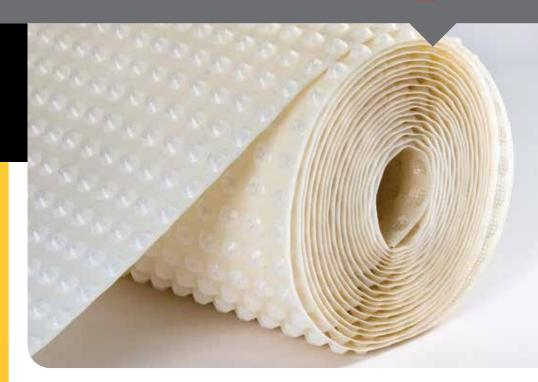
**CM8 Cavity Drain Mesh Membrane** is a 8 mm studded membrane incorporating a tough HDPE mesh lathing welded to the front face, allowing the direct application of various plaster finishes, adhesive 'dabs' and plasterboards and delivering a grade 3 environment to BS8102:2009 and NHBC Chapter 5.4.
