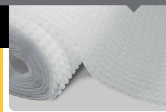
**CM8 Cavity Drain Membrane** is an 8 mm studded membrane, suitable for Type C waterproofing and delivering a grade 3 environment to BS8102:2009 and NHBC Chapter 5.4. CM8 is available in both 500g or 700g densities. We recommend using the CM8 HD700 when a heavier, denser membrane is deemed necessary by the Wykamol Technical Department. Please always take advice from our Technical Experts when making product selections.
