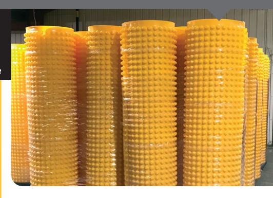
**The CM20 High-visibility Yellow Cavity Drain Membrane** is a 20mm studded membrane, suitable for Type C waterproofing and delivering a grade 3 environment to BS8102:2009 and NHBC Chapter 5.4. CM20 Yellow is the highest drainage capacity membrane in the Wykamol Waterproofing range.
