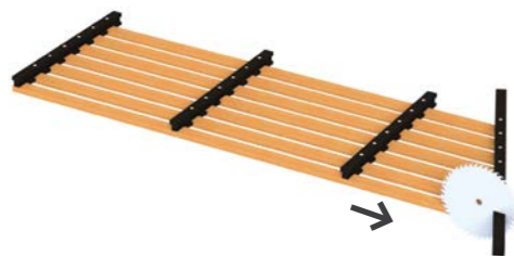
Step 5: Cut the surplus of the cutting profile
