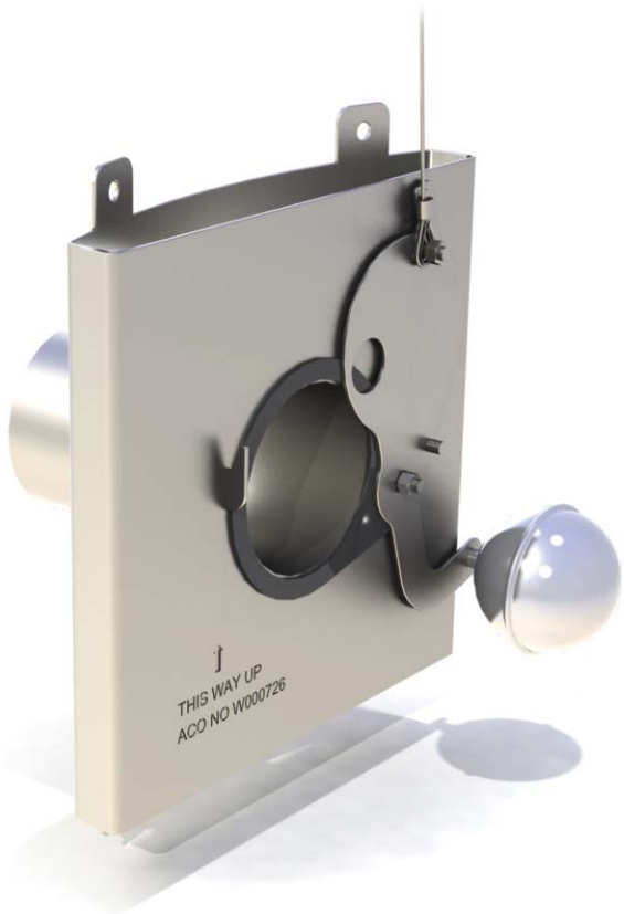
ACO Q-Plate with remote draindown and bypass recommended for all orifice apertures less than 100mm
